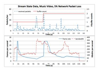
Fig. 3. Stream state data collected by our instrumented media player for a music video experiencing 5% network packet loss and 100ms network delays.
