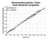
Fig. 2. The cumulative number of retransmitted packets for a portion of a UDP video stream, measured at two different clients under moderate congestion. The solid black lines connecting the two plots show the point-to-point matching performed by DTW, illustrating that the closest matches between points do not always line up exactly in time.
